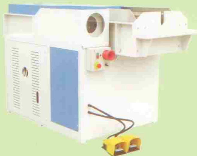
KIT IDRAULICO TRAFILATURA TUBO PER FEDI MOD. VM/KTF 10 HYDRAULIC DRAWING BENCH KIT MOD. VM/KTF 10
